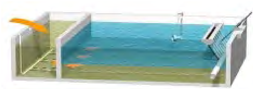
Figure 42. SBR Tank (Sanitaire)
