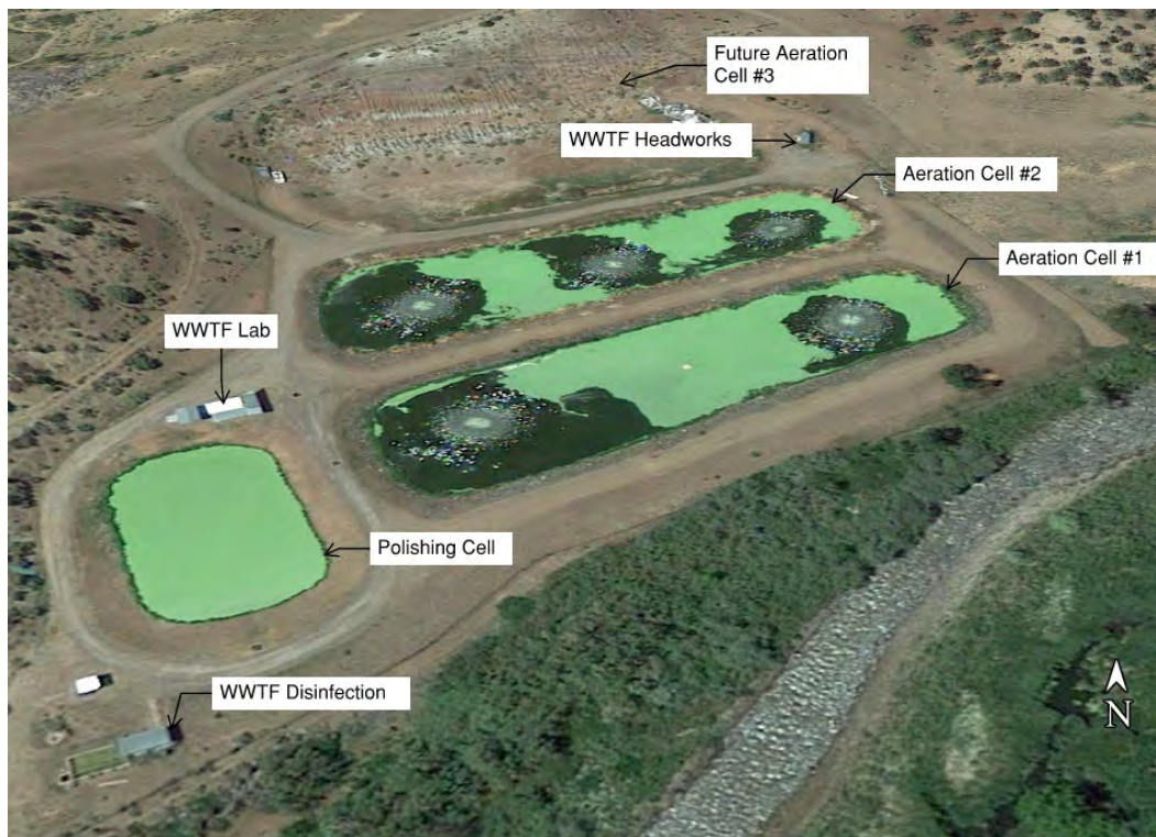
Figure 5. WWTP Site Layout
